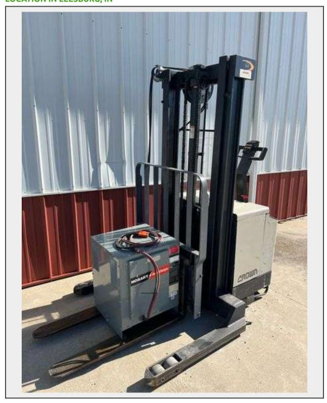
Crown 40WTL Walkie Stacker 42" Manual Adjust Forks, 5" Wide Forks, Tilt, 2-Speed, Double Mast 130" Lift Height, 4,000 lb. Lift Capacity, Hobart Accu-Charger 24V Battery Charger, In working condition - PICK UP AT ALTERNATE LOCATION IN LEESBURG, IN
