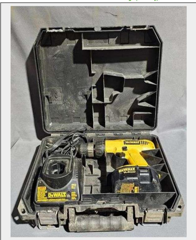
DeWalt DW954 3/8" (10mm) VSR cordless drill with adjustable clutch. Includes a 14.4V nickel-cadmium battery, DW9118 charger (7.2V–14.4V compatible), and the original hard-sided case for storage.
