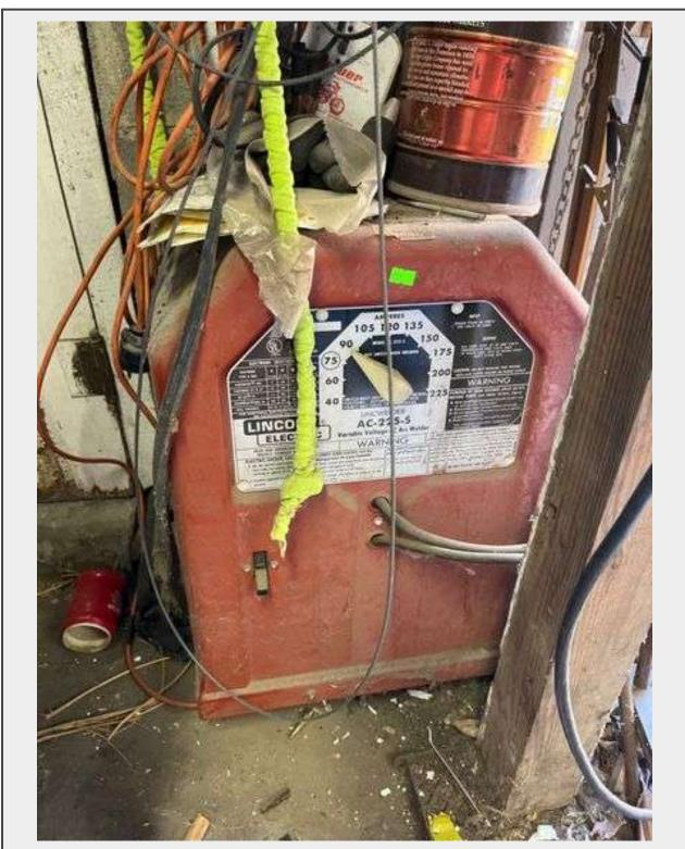
Lincoln Electric AC-225-S variable voltage arc welder, NEMA Rating Class III (20). The panel includes labeled amperage settings ranging from 40-225 amps for various welding applications.
