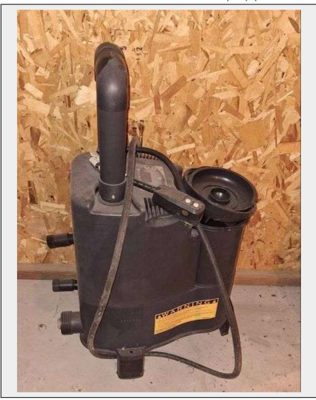
Comfort Line Products Model CL250-C electric spa equipment, designed for use with hot tubs, spas, and associated systems. Runs on 120 volts, 12 amps, 60 hertz. Manufacturer and safety information detailed on the attached label. Features include an attached hose, control mechanism, and operational components. Manufactured on 08/06/07.
