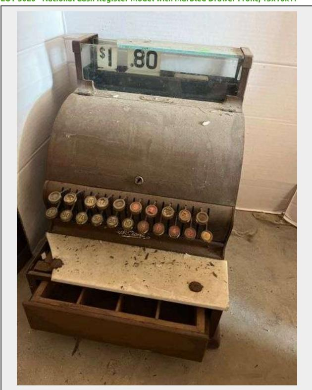
National cash register featuring a marbled drawer facade, multiple mechanical push buttons for various denominations, and a built-in glass display at the top. Includes dollar and cent counters, a customer counter, and a sale ledger. Dimensions are 13x16x17.
