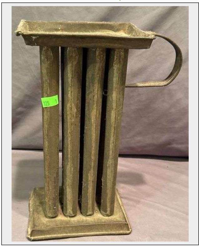
Metal candle mold designed with 12 vertical tubes for forming candles. Features a flat top with openings for pouring wax and a sturdy handle for ease of use. The mold includes a rectangular base for stability. Measurements: 10"x6"x4.5".
